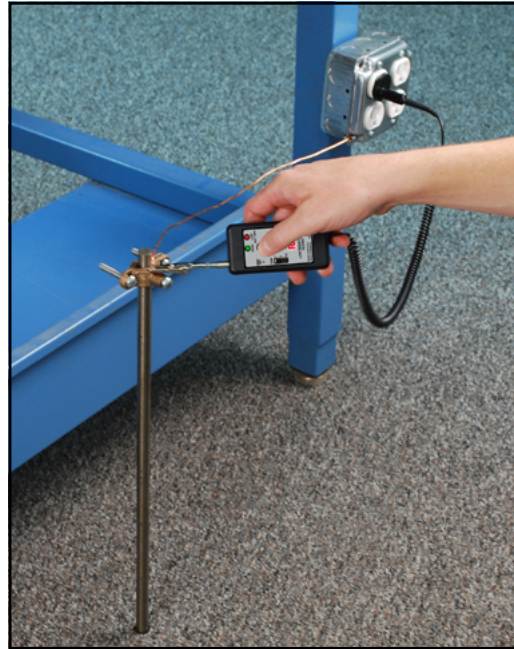
Figure 4. Testing auxiliary ground with the 126-8850 tester
