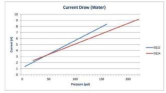
Pressure shown is the not to exceed value. All MG2000 pump variants are capable of more than the indicated figure but exceding this may result in damage to the pump.
