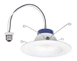
The Contractor Series RT5/6 is a 5" and 6" compatible LED recessed downlight kit creating high performing white light and is optimized for new construction and retrofit applications. Installation is done quickly and easily in most standard 5" or 6" Insulated Ceiling (IC) housings, Airtight (AT) housings and non-IC housings.
