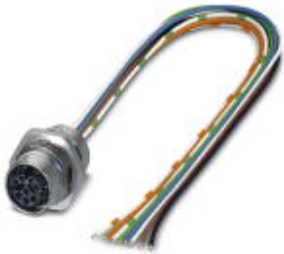
Flush-type socket, Universal CAT5 (IEC 11801:2002), 8-position, Socket, M12-SPEEDCON, Y - hybrid, Rear mounting, M16 x 1.5, Contacts with connected litz wires, cable length: 0.5 m
