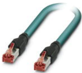
Assembled Ethernet cable, shielded, 4-pair, 26 AWG stranded (7-wire), RAL 5021 (water blue), RJ45 plug/IP20 to RJ45 plug/IP20, line, length: 2 m
