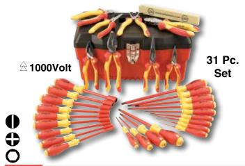
31 Pc. Pliers & Screwdriver Set. Insulation According to VDE 0682/part 201, EN/IEC 60900, ASTM F-1505, NFPA70E & CSA, A up to 1000 volt. Individually Tested. Pliers drop-forged from special tool steel, individually high frequency induction hardened, chrome/nickel plated, mirror-polished. Set includes 6ft. Fiber glass folding ruler.
