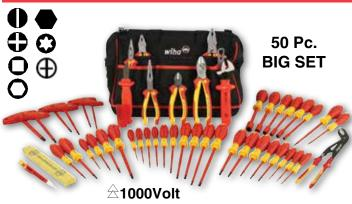
50 Piece Insulated Tool Set. Insulation According to VDE 0682/part 201, EN/IEC 60900, ASTM F-1505, NFPA70E & CSA, up to 1000 volt. Individually Tested. Pliers drop-forged from special tool steel, individually high frequency induction hardened, chrome/nickel plated, mirror-polished. Cushion Grip Insulated handles. Canvas tool bag.
