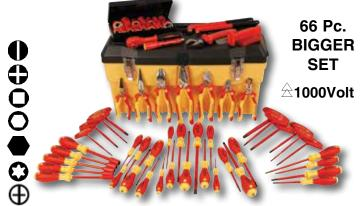
32876 66 Pc. Master Electrician's Set. Insulation According to VDE 0682/part 201, EN/IEC 60900, ASTM F-1505, NFPA70E & CSA, up to 1000 volt. Individually Tested. Pliers drop-forged from special tool steel, individually high frequency induction hardened, chrome/nickel plated, mirror-polished.
