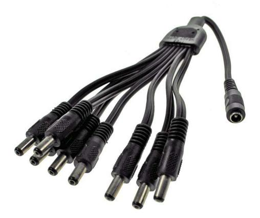
**DC Extension Splitter Cable** – From a 2.1mm DC input socket and terminates with 8 x 2.1mm DC connectors. They enable a single output to be split allowing a number of units to be powered from a single source. All cables are manufactured using 20AWG cable.
