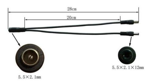
**DC Extension Splitter Cable** – From a 2.1mm DC input socket and terminates with 2 x 2.1mm DC connectors. They enable a single output to be split allowing a number of units to be powered from a single source. All cables are manufactured using 20AWG cable.
