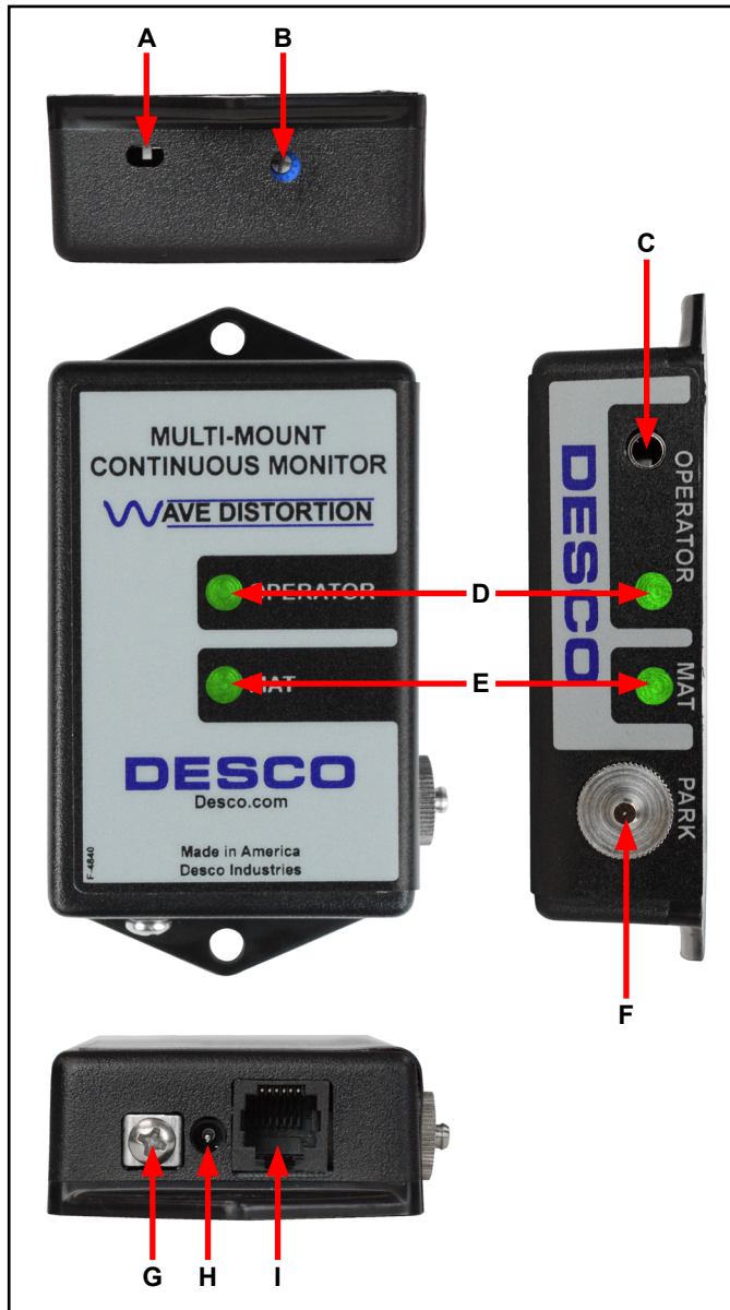
Figure 5. Multi-Mount Monitor features and components
