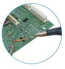
Quickly removes excess solder
