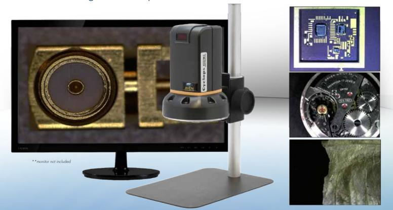
This innovative inspection scope connects directly to an HD monitor through a convenient 1080p HDMI output allowing operators to view high quality magnified images while looking straight ahead at a large screen, rather than hunching over narrow eyepieces. A large working distance and 30 LEDs that can be adjusted for intensity allow examination of objects of various sizes. Magnification ranges up to 132x on a 21.5" HD monitor.
