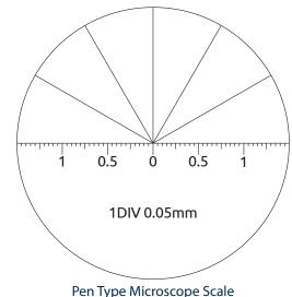
Etched into the eyepiece with graduations of 0.05mm 26800C-552 & 26800C-553
