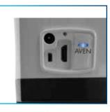
USB and HDMI outputs. Connect to your monitor for lagfree 1080p inspection with the HDMI port. Or use the USB port to connect to your PC.
