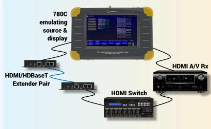
**Example Network Test Setup**
