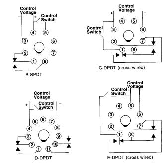
The **Duplexor** is used in control panels where **two loads** are required to alternate to provide equal run time on the loads. The alternating action is initiated by a control switch, which is common with one side of the control voltage. The output contacts will change states each time the control switch is opened, thus alternating the two loads. The LED indicators show the position of the output relay.
