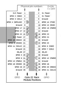
Place this overlay over your Pi's GPIO pins for a handy mapping reference. You can download the template from developer.opto22.com.
