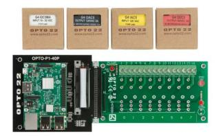
5. Remove an I/O module from its box and carefully install it in position 0 on the board. Secure it with its integral screw.
