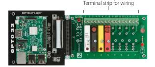
7. Follow "Field Wiring Diagrams" on page 4 to wire realworld sensors and devices to the mounting rack.
