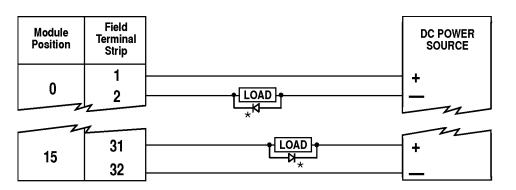
\*Note: Commutation diode must be used on inductive loads. Typically, use diode 1N4005
