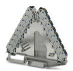
Potential distributors, Nom. voltage: 250 V, Nominal current: 17.5 A, Cross section: 0.14 mm² - 2.5 mm², AWG: 14 - 26, Connection type: Push-in connection, Number of positions: 2, Number of connections: 32, Width: 8.3 mm, Length: 100 mm, Color: gray, Color of connection elements: blue, Assembly: NS 35/7,5, NS 35/15
