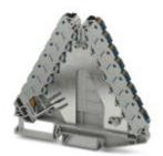
Potential distributors, with option to supply up to 6 mm², Nom. voltage: 250 V, Nominal current: 17.5 A, Cross section: 0.14 mm² - 2.5 mm², AWG: 14 - 26, Connection type: Push-in connection, Number of positions: 2, Number of connections: 29, Width: 8.3 mm, Length: 100 mm, Color: gray, Color of connection elements: blue, Assembly: NS 35/7,5, NS 35/15
