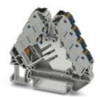
Potential distributors, with option to supply up to 6 mm², Nom. voltage: 250 V, Nominal current: 17.5 A, Cross section: 0.14 mm² - 2.5 mm², AWG: 14 - 26, Connection type: Push-in connection, Number of positions: 2, Number of connections: 13, Width: 8.3 mm, Length: 64 mm, Color: gray, Color of connection elements: blue, Assembly: NS 35/7,5, NS 35/15
