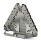
Potential distributors, with option to supply up to 6 mm², Nom. voltage: 250 V, Nominal current: 17.5 A, Cross section: 0.14 mm² - 2.5 mm², AWG: 14 - 26, Connection type: Push-in connection, Number of positions: 2, Number of connections: 29, Width: 8.3 mm, Length: 100 mm, Color: gray, Color of connection elements: black, Assembly: NS 35/7,5, NS 35/15
