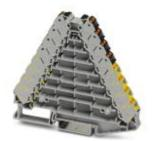
Potential distributors, Nom. voltage: 250 V, Nominal current: 17.5 A, Cross section: 0.14 mm² - 2.5 mm², AWG: 14 - 26, Connection type: Push-in connection, Number of positions: 2, Number of connections: 32, Width: 8.3 mm, Length: 100 mm, Color: gray, Color of connection elements: black, yellow, Assembly: NS 35/7,5, NS 35/15
