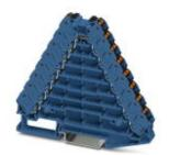
Potential distributors, Nom. voltage: 250 V, Nominal current: 17.5 A, Cross section: 0.14 mm² - 2.5 mm², AWG: 14 - 26, Connection type: Push-in connection, Number of positions: 2, Number of connections: 32, Width: 8.3 mm, Length: 100 mm, Color: blue, Color of connection elements: black, Assembly: NS 35/7,5, NS 35/15
