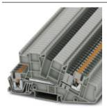
Installation level terminal block, Push-in connection, Cross section: 0.14 mm² - 4 mm², AWG: 26 - 12, Width: 5.2 mm, Color: gray, Mounting type: NS 35/7,5, NS 35/15
