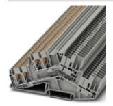
Double-level terminal block, Connection type: Push-in connection, Cross section: 0.14 mm<sup>2</sup> - 4 mm<sup>2</sup>, AWG: 26 - 12, Width: 5.2 mm, Color: blue, Mounting type: NS 35/7,5, NS 35/15
