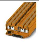
Component terminal block, with integrated 1N4007 diode, nom. voltage: 800 V, nominal current: 0.5 A, connection method: Push-in connection, number of connections: 4, cross section:0.14 mm<sup>2</sup> - 4 mm<sup>2</sup>, AWG: 26 - 12, width: 5.2 mm, color: orange, mounting type: NS 35/7,5, NS 35/15
