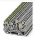
Sensor/actuator terminal block, with integrated diode, Connection method: Spring-cage connection, Cross section: 0.08 mm² - 4 mm², AWG: 28 - 12, Width: 5.2 mm, Color: gray, Mounting type: NS 35/7,5, NS 35/15
