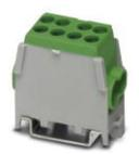
Trunk line branch terminal, nom. voltage: 400 V, nominal current: 101 A, connection method: Screw connection, Screw connection, number of connections: 4, number of positions: 1, cross section:1.5 mm² - 25 mm², AWG: 8 - 2, width: 23 mm, color: green, mounting type: NS 35/7,5, NS 35/15
