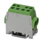
Trunk line branch terminal, nom. voltage: 400 V, nominal current: 125 A, connection method: Screw connection, Screw connection, number of connections: 4, number of positions: 1, cross section:10 mm² - 35 mm², AWG: 8 - 2, width: 27 mm, color: green, mounting type: NS 35/7,5, NS 35/15
