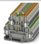
Knife disconnect terminal block, With test socket screws for insertion of test plugs, Connection type: Screw connection, Cross section: 0.14 mm² - 4 mm², AWG: 26 - 12, Nominal current: 16 A, Nominal voltage: 400 V, Length: 80.1 mm, Width: 5.2 mm, Color: gray, Assembly: NS 35/7,5, NS 35/15
