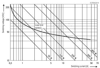
Load limit curve 1: arc extinguishes during transit time (changeover contact). Load limit curve 2: safe shutdown, no stationary arc (make contact). Load limit curves measured with low inductive resistors verified for 1000 switching events.
