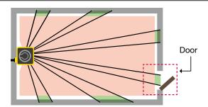
Reference monitoring function ensures safety by detecting the positional change of SE2L or reference boundary, such as a door's opening/closing status.
