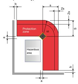
Maintain the distance "a" shorter than the minimum detection width. To prevent unwanted detection, maintain the distance "b" 100mm.
