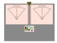
An SE2L can monitor two separate hazardous areas to stop machines when detecting the access of humans. No reflective sensor is necessary, thus eliminating the need of optical axis alignment. Can replace two light curtains.
