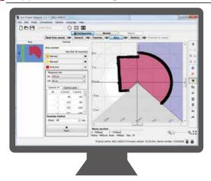
Teaching function enables automatic area configuration by referring to obstacles such as walls and columns. Area can be configured easily even with complicated background.
