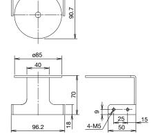
Used to protect the optical window in combination with base mounting bracket or rear mounting bracket.
