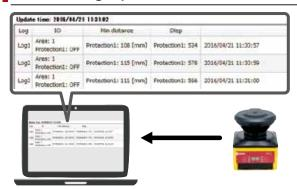
Operational status is displayed on the SE2L. It can also be displayed on PC to monitor errors and data log for easy trouble shooting.
