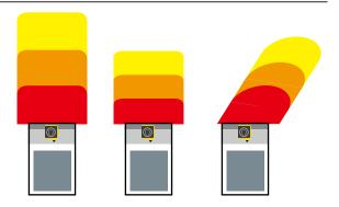
A maximum of 32 area patterns can be configured/ switched according to the mobile application such as AGV, ensuring the optimum protection in various applications.
