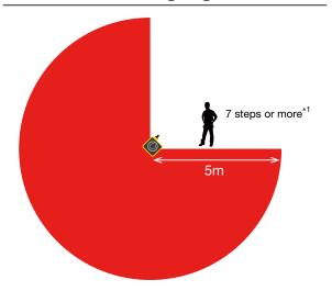
One SE2L protects a wide area (270° and 5m) and can be used in a variety of applications such as large sized systems or long conveyor lines.
