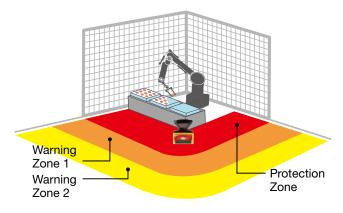
Warning zones 1 and 2 are set around the protection zone to send alarms to prevent humans or objects from entering the hazardous area and stopping the machine. By detecting humans or objects in the protection zone, the OSSD signal switches from ON to OFF. Also, when humans or objects are detected in the warning zone, WARNING signal switches from ON to OFF.
