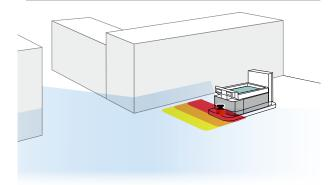
During safety protection, the SE2L can send out distance measurement data through the Ethernet port, in order to obtain the data of the obstacles.
