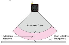
\* Additional distance: the distance required to operate the SE2L under high reflective background
