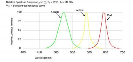
Fig.1 Relative Luminous Intensity vs. Wavelength
