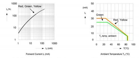
Fig.2 Relative Luminous Intensity vs. Forward Current
