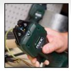
**Trigger Design:** The innovative trigger reduces hand force from 53 lbs to 6 lbs and allows a dramatic reduction in fatigue rates and risk of ergonomic injury.
