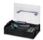
Tool for processing ferrules according to DIN 46228-4, 0.5 mm² to 2.5 mm², equipped with pressure lock, cutting, stripping, twisting, and crimping unit, with three magazines including a strip each of ferrules from 0.5 mm² ... 2.5 mm², packaged in a robust plastic case
