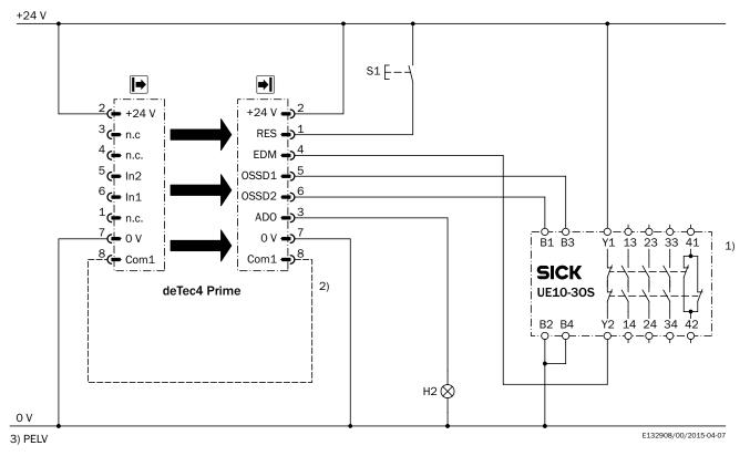
① Output circuits. These contacts must be incorporated into the control such that the dangerous state is brought to an end if the output circuit is open. For categories 4 and 3, they must be incorporated on two channels (x, y paths). Single-channel incorporation into the control (z path) is only possible with a single-channel control and taking the risk analysis into account.
