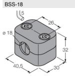
6901320 Mounting clamp for smooth and threaded barrel sensors; material:
