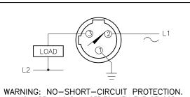
ALWAYS WIRE A LOAD IN SERIES WITH THE SENSOR.
