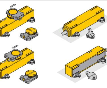
Extensive mounting accessories provide various options for installation.
