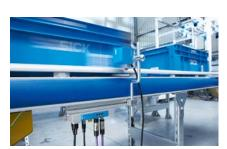
The CLV6xx bar code scanners, from the CLV69x with oscillating mirror for pallet identification to the CLV615 for reading totes, can be used across the whole logistics chain.
