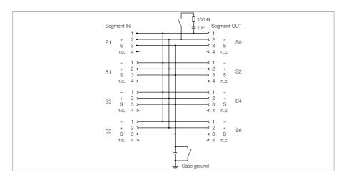
The 6-channel junction box JBBS-49-E613/3G is designed for FOUNDATION™ fieldbus systems.
