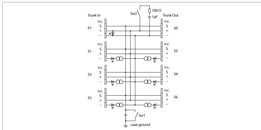
The 6-channel Ex junction box JBBS-48SC-T615B/EX is designed for PROFIBUS-PA systems.
