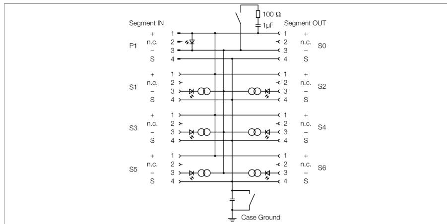
The 6-channel Ex junction box JBBS-48SC-E613/EX is designed for PROFIBUS-PA systems.
