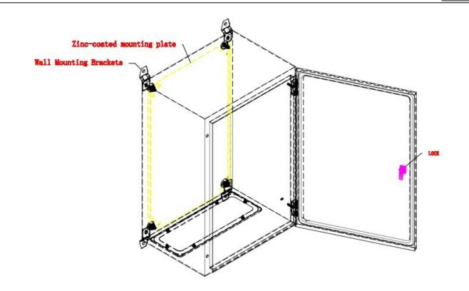
**Application:** A mild steel IP66 industrial wall box suitable for housing electronic and electrical equipment in demanding environments, where the area is prone to frequent hosing or generally wet conditions.
