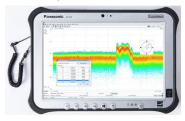
When purchased from Tektronix, the FZ-G1 includes pre-loaded SignalVu-PC software, with custom-programmed display settings and front-panel buttons to optimize the SignalVu-PC experience.
