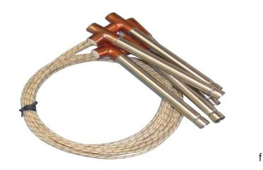
Air heaters feature an open coil of high temperature resistance wire electrically isolated in a stainless steel sheath. Because the air being heated passes directly over the resistance wire, maximum heat transfer efficiency is achieved. Ar heaters are used for heat staking, plastic welding, laminating, drying, heat sealing, and any other operation where air needs to be heated up 500°C
