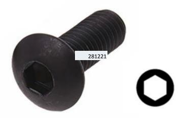
Button Head Socket Screws are designed for light duty. They have a similar thread design as a Socket Cap Screw although the dome shaped head is wider and has a lower profile than a Socket Cap Screw, presenting an aesthetic appearance to an assembly. These fasteners are ideal when a wider bearing surface is required.
