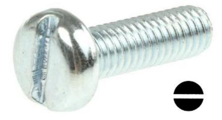
Pan head machine screws similar to oval head machine screws have rounded sides, the difference being that pan head machine screws have a flat top rather than rounded. The slotted drive is a popular driving method with this type of fastener for ease of assembly. Machine screws can be used in pre-tapped holes or used with conforming nuts and washers in through holes.
