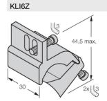
Mounting bracket for mounting magnetic field sensors on tie-rod cylinders; cylinder diameter: 50...125 mm; material: Aluminum
