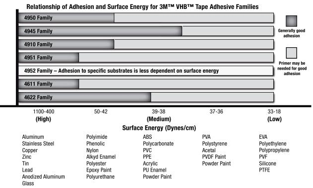
NOTES: There are a wide variety of formulations, surfaces finishes and surface treatments available on substrate materials which can affect adhesion. This chart is intended to provide only a rough estimate of the adhesion levels which can be expected on some common materials relative to a reference surface such as aluminum.
