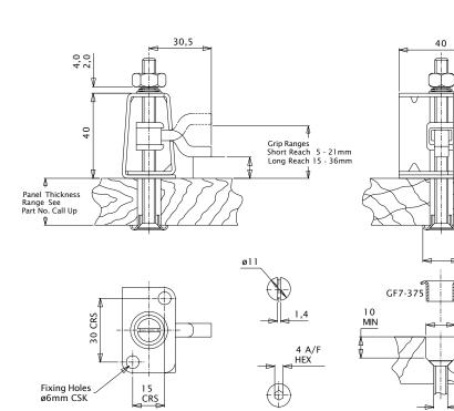
Prepare panel (drill 11mm hole). Assemble grommet onto screw, insert screw through panel hole and use to locate housing to panel by 4mm (No.8) countersunk screws (not supplied).
