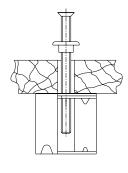
STAGE 2 Locate and thread pawl onto screw (pawl may be fitted either way dependant on support thickness) continue threading through the pawl until the screw head seats in the panel hole, and the tip protrudes through the bottom of the housing. Locate the friction spring over the end of the screw (larger end against the housing) and secure assembly with locknut, so the spring is compressed as assembly stage 2, to within 2-4mm gap.
