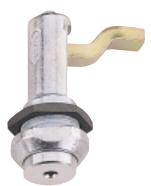
The DP 140 Adjustable Pawl Latch is designed for use on air handling units, electronic cubicle doors, passenger transport valance doors and in the machine tool and sheet metal industries. The pawl finger travels up a threaded spindle and operation is achieved by a quarter clockwise turn to lock; the head remaining flush with the escutcheon when adjusted to the fully locked position. A quarter turn anti-clockwise releases the latch, the head ejecting to signal its unlocked state.
