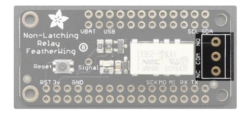
Both Wings have the same output, a 3-pin 3.5mm terminal block. The COM pin is what you should connect the signal you're planning to switch. If the relay is unset, the NC pin (Normally Connected) is mechanically connected to COM. NO (Normally Open) is mechanically disconnected.
