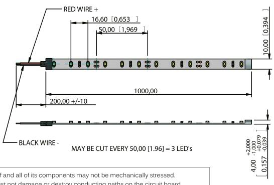
The strip itself and all of its components may not be mechanically stressed. Assembly must not damage or destroy conducting paths on the circuit board. Correct electrical polarity needs to be observed, wrong polarity may destroy the strip. When mounting on a metallic or otherwise conductive surfaces, there needs to be electrical isolation points between strip and the mounting surface.
