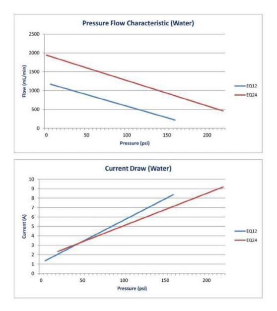
Pressure shown is the not to exceed value. All MG2000 pump variants are capable of more than the indicated figure but exceeding this may result in damage to the pump.
