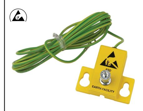
"The protection of ESDS [ESD sensitive item] is accomplished by providing a ground path to bring ESD protective materials and personnel to the same electrical potential. All conductor and dissipative items in the environment, including personnel, shall be bonded or electrically connected to a known ground or common connection point [Earth Bonding Point]." [CLC/TR 61340-5-2:2008 User guide clause 4.4.1 Grounding/bonding systems Introduction]
